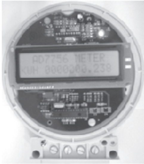
Figure 2. Final Implementation of the ADE7756 Meter
